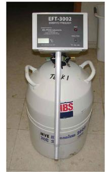
**1. Slowly insert freezer into liquid nitrogen "LN<sub>2</sub>" tank**
