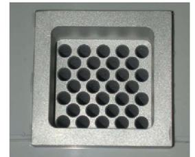
**4. Place cap on freezing chamber.** The controller will automatically allow the freezing chamber to cool down to the start temperature ( -6.5C). This will take approximately 45 minutes from room temperature. Once the temperature has stabilized for 3 minutes you may place the prepared embryos into the freezer with the straw ID extending above the chamber.
